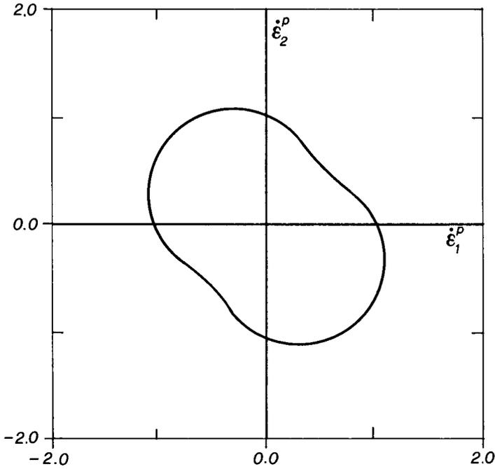
Fig. 3. – Plot representing the contour line  $D(\dot{\epsilon}_1^p, \dot{\epsilon}_2^p)/\sigma_y = 1$  for a material having  $f = \sigma_1^2 + \sigma_2^2 - \sigma_1\sigma_2 + -\sigma_y^2 \leq 0$  as yield function and  $g = \sigma_1^2 + \sigma_2^2$  as plastic potential function.
