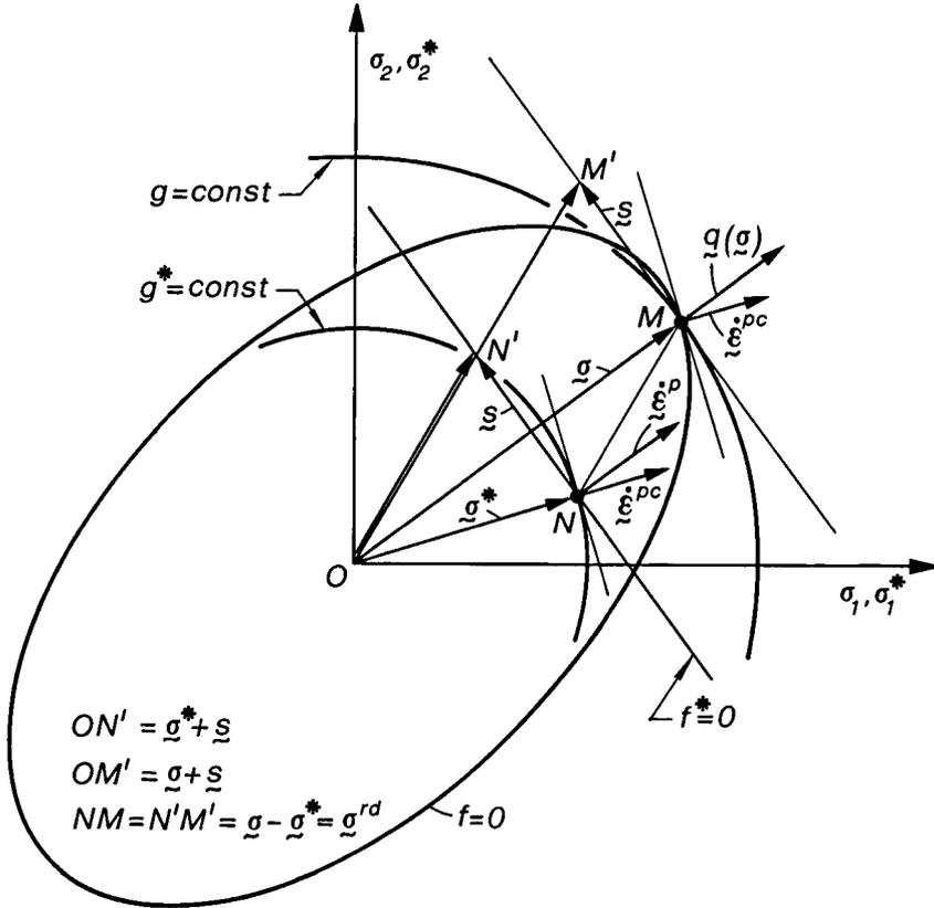
Fig. 2. – Non-associative material behaviour described as a fictitious composite material with two associative plastic constituents in the superposed two-dimensional stress and strain spaces.
