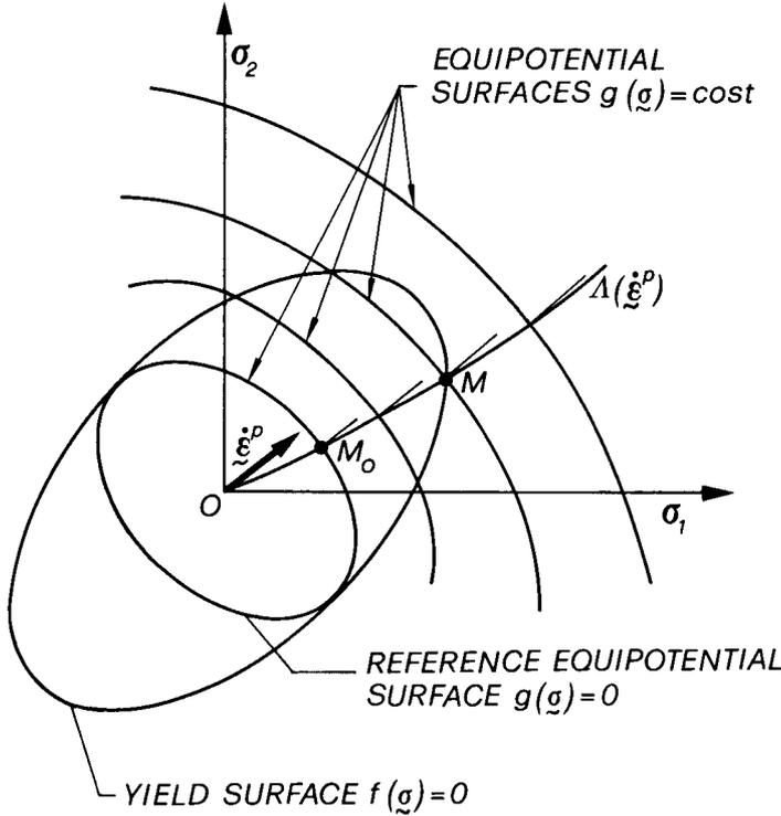
Fig. 1. - Yield surface  $f(\sigma_1, \sigma_2) = 0$  and equipotential surfaces  $g(\sigma_1, \sigma_2) = \text{const}$  in two-dimensional stress space.
